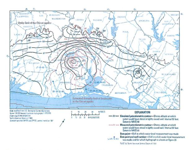
Figure 5-5 – Simulated and measured water level elevation contours in the Chicot Formation, 2009.
