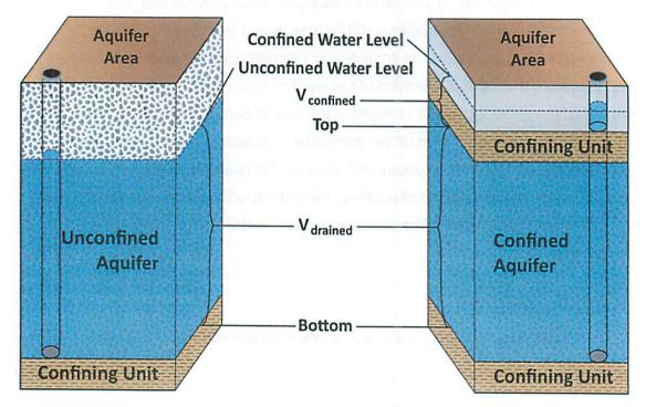
FIGURE 1. SCHEMATIC GRAPH SHOWING THE DIFFERENCE BETWEEN UNCONFINED AND CONFINED AQUIFERS.
