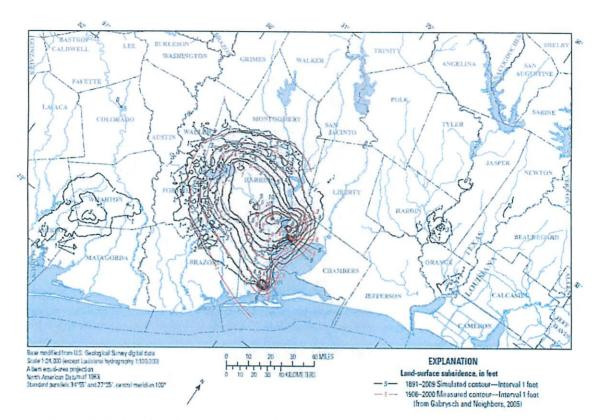
Figure 5-8 – Simulated and measured subsidence contours occurring in the Gulf Coast Aquifer System, 2009.
