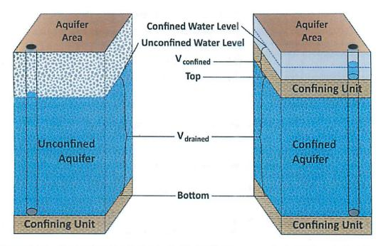
Figure 5-21 – Illustration of relevant hydrological features on which TERS analysis is based
