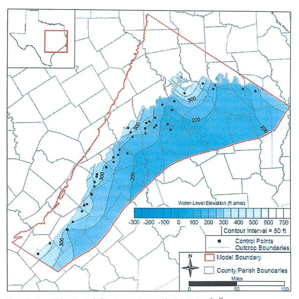
Figure 5-11 – 1999 estimated elevation contours in the Sparta Aquifer<sup>45</sup>
