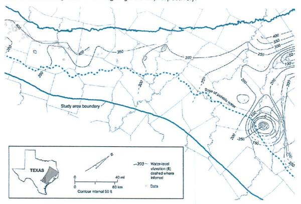
Figure 5-9 - Water level elevation contours in the Carrizo Sand Aquifer based on water level measurements from  $1987-1990^{43}$
