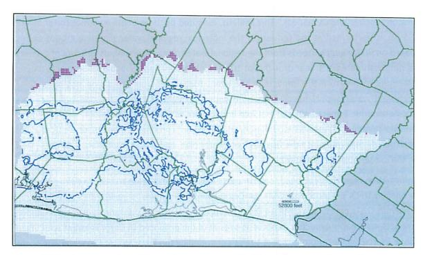
Figure 5-25 – Contours of subsidence from Northern Gulf Coast GAM Run 2 using SUB package for predictive period of 2010-2070.
