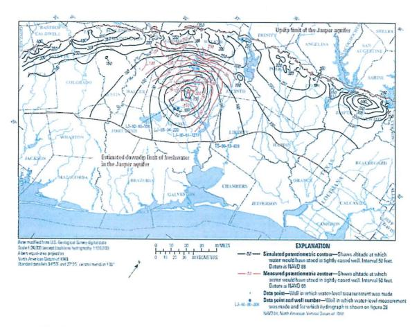
Figure 5-7 – Simulated and measured water level elevation contours in the Jasper Formation, 2009.
