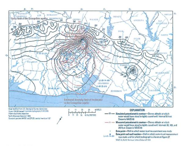
Figure 5-6 – Simulated and measured water level elevation contours in the Evangeline Formation, 2009.
